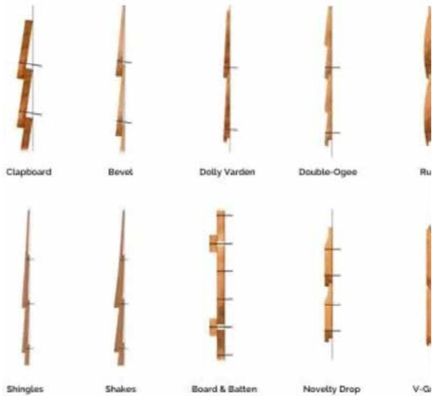
Figure 3-23. Examples of common siding profiles, to be matched as closely as possible. Source: Scott Sidler, "The Ultimate Guide to Wood Siding," The Craftsman Blog, updated June 1, 2020, <https://thecraftsmanblog.com/the-ultimate-guide-to-wood-siding/>.
