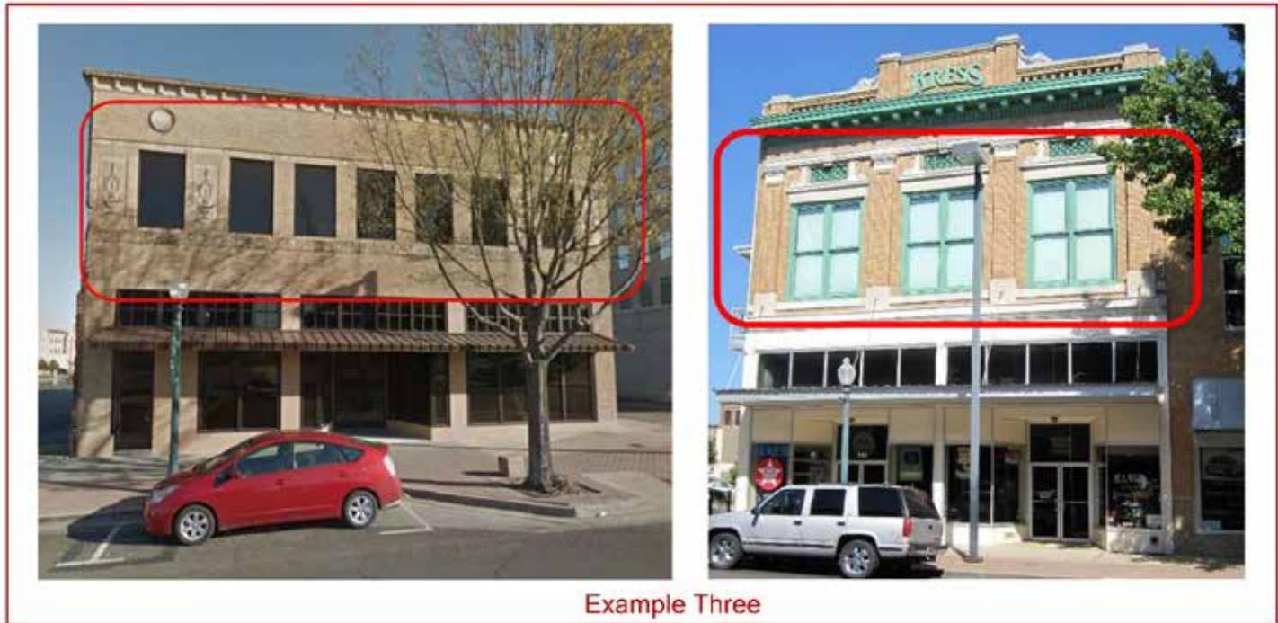
Figure 3-36. Examples of **inappropriate** new shutters improperly sized to fit the original window openings. Source: Scott Sidler, "All About Wood Shutters," The Craftsman Blog, published October 8, 2020, <https://thecraftsmanblog.com/all-about-wood-shutters/>.
